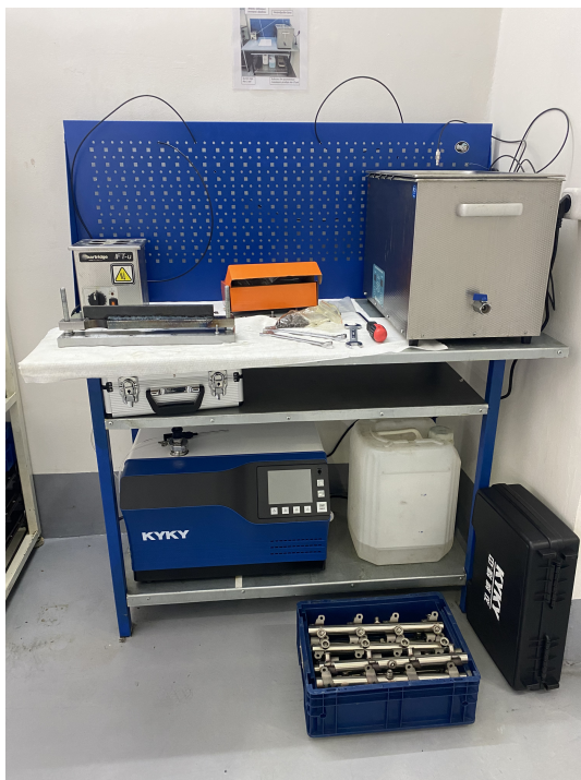
Figure 3 — Workstation with a helium leak detector and test fixtures. Access to connections and controls must be provided when arranging the station.
